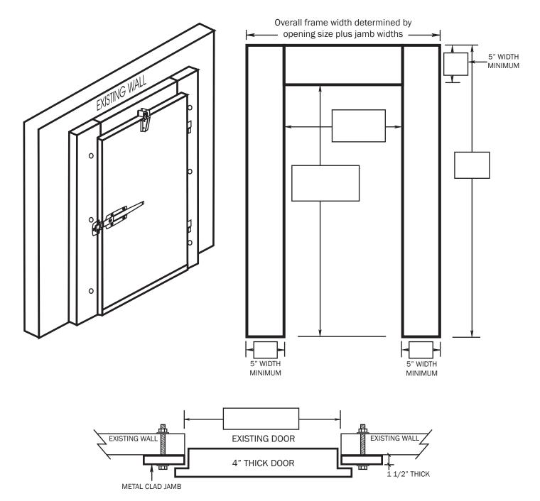
This door and metal clad jamb bolts through the existing wall. All doors come with standard hardware including door closer, cam lift side mounted hinges, and a positive latch with offset strike.
